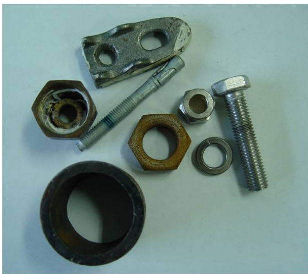
Fig. 18. Radioactive contaminants supplied from Unit 1 of the Wolsung and Unit 2 of the Kori Nuclear Power Plants during overhaul periods.
