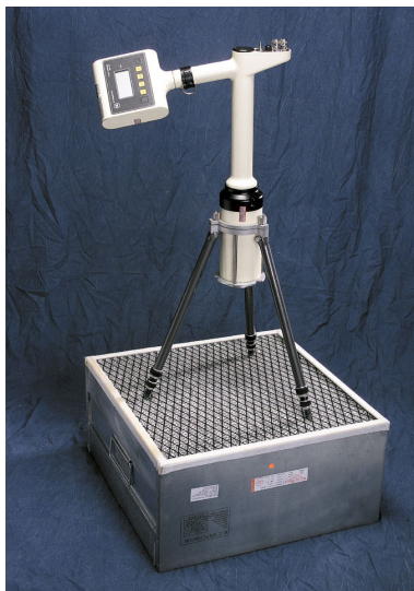
Fig. 2. LRGS positioned for HEPA filter monitoring
