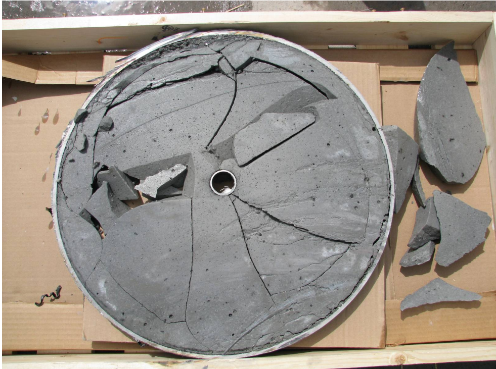
Fig. 12. Cracking in the mid-plane in CWF1
