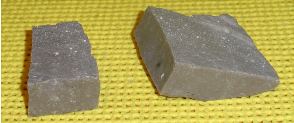
Fig. 4. Second (left) and First (right) Failed Sections
