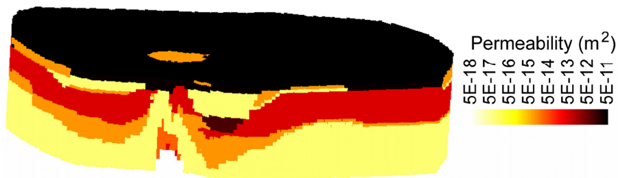
Fig. 5. Gorleben model. Block diagram. Vertical exaggeration ratio 12:1
