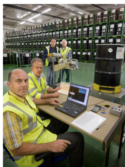
Fig. 1. SNAP assay system monitoring a 200l waste drum on a rotating turntable
